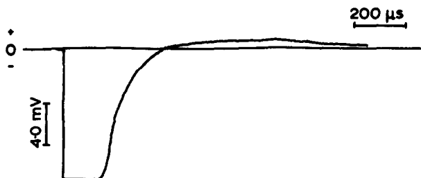
Fig. 8. The Demer photovoltages of D9/Si with D9 facing light.
