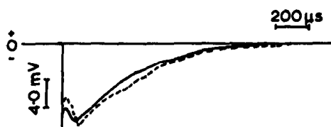
Fig. 3. Dember photovoltages of: (·····) Si/NTCC + TNC-3; (—) Si/NTCC + TNC-4 with Si facing light.
